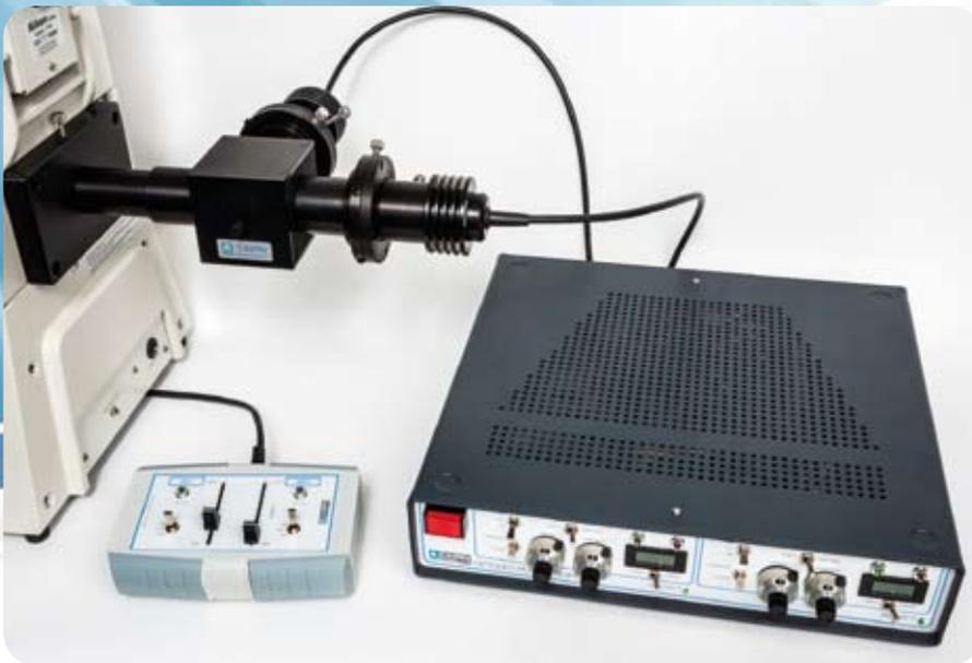
High intensity LEDs are now available across the visible spectrum extending into both the ultraviolet and infrared. Their longlife, high stability, variable intensity and lower power consumption make them ideal for both fluorescence and transmitted light microscopy. The Cairn OptoLED system has been designed to best exploit this new technology whilst maintaining compatibility with arc lamp and laser illumination sources.
